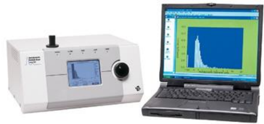
Figure 9. TSI Aerodynamic Particle Sizer (APS) model 3321 used to measure total particle concentration and particle size distribution of the challenge bioaerosol. It has a range of 0.54-20.0 μm aerodynamic diameter, with 1 particle/L detection limits.
