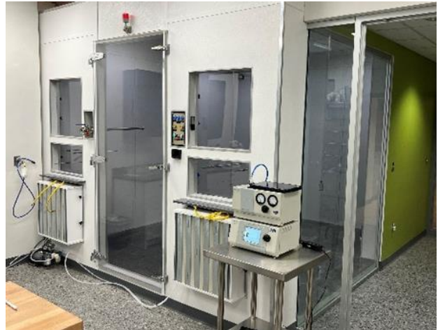
Figure 3: The 30 m 3 bioaerosol testing chamber at ARE Labs adheres to AHAM AC-5 standards and ASHRAE 241 criteria. The chamber is equipped with HEPA filtered air in/out, multiple bio aerosol sampling ports, decontamination, and pressure balance.
